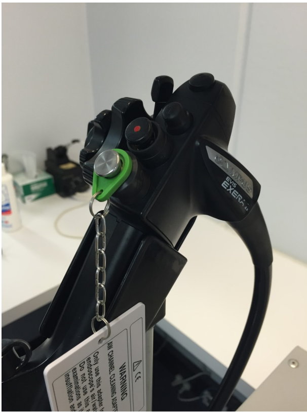
Attach Air / Water channel cleaning adapter. Press Air / Water cleaning button for 10 seconds, then release for 10 seconds.
