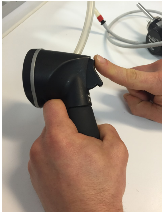
Before pumping air into the endoscope be certain the leakage tester valve is closed by pressing the button in at the top.
