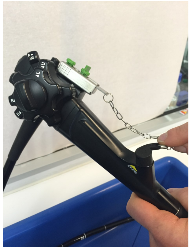
All suction cleaning adapter should be connected to the biopsy channel and the valve ports, this is achieved by pushing downward and sliding the metal casing over the port locking it in place.
