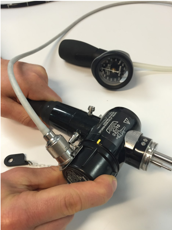
Place the endoscope on a work bench and attach soaking cap with the leakage tester connected to perform a dry leak test.
