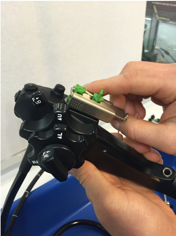
All suction cleaning adapter should be connected to the biopsy channel and the valve ports, this is achieved by pushing downward and sliding the metal casing over the port locking it in place.
